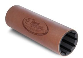
Johnson Cutless® Non-Metallic Sleeve Bearings feature a dense structure of engineered reinforced thermoset plastic. The specially compounded Nitrile Rubber is securely bonded to the shell with all tolerances maintained for proper lubrication. Being non-corrosive and inherently resistant to all known chemicals, oil and grease, as well as being anti-electrolytic, the Johnson Cutless® Non-Metallic Sleeve Bearings are ideally suited for installations wherever corrosion or electrolysis is a problem.
